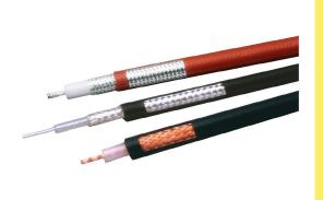
The RG-213 coax cable also has a frequency range of up to 1 GHz and an impedance of 50 or 75 ohms. It has a solid copper conductor, a polyethylene dielectric, and a braided shield.
